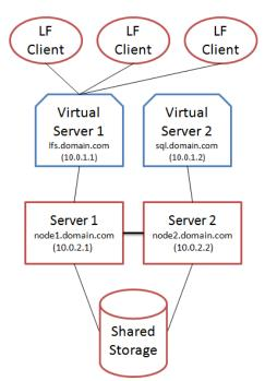
In this scenario, a Laserfiche Server and a Microsoft SQL Server instance are still installed on *both* **Server 1** and **Server 2**. However, before failover, the virtual servers each run on a separate node: **lfs.domain.com** forwards to **node1.domain.com** and **sql.domain.com** forwards to **node2.domain.com**.
