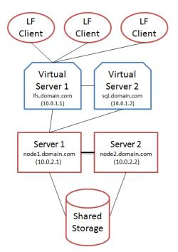
In this scenario, a Laserfiche Server and a Microsoft SQL Server instance are installed on both **Server 1** and **Server 2**. These two machines are clustered together to create:
